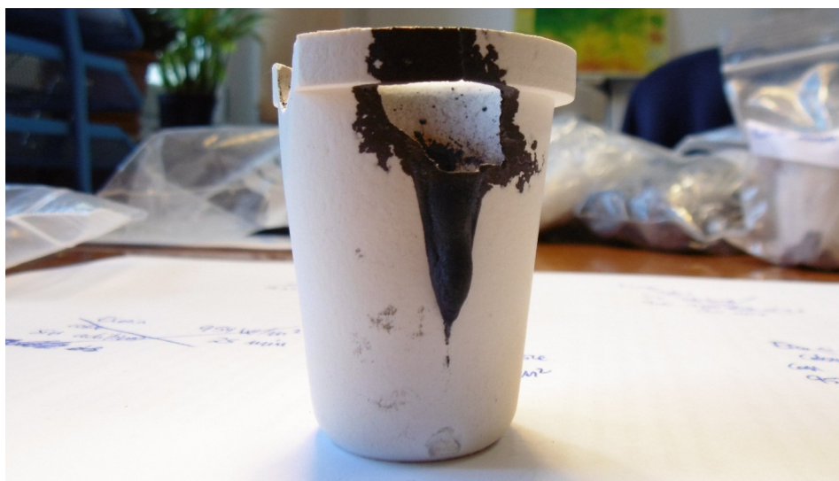
Fig. 4. The crucible (tabular alumina), where the temperature was high enough to melt the walls.
