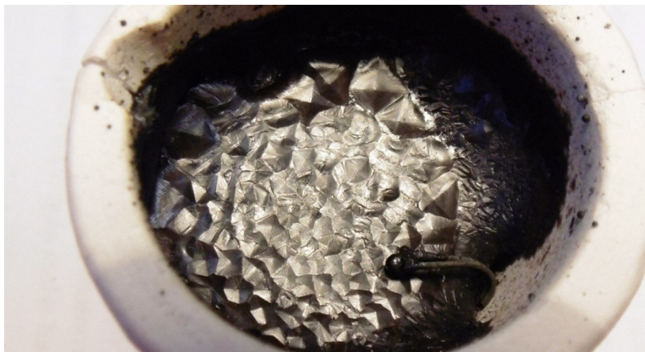
Fig. 6. A sample of BOF slag after the treatment with concentrated solar energy. Good crystallization can be observed.
