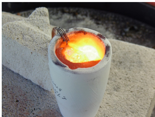
Fig. 4. Presence of molten phase in the crucibles during the experiments.
