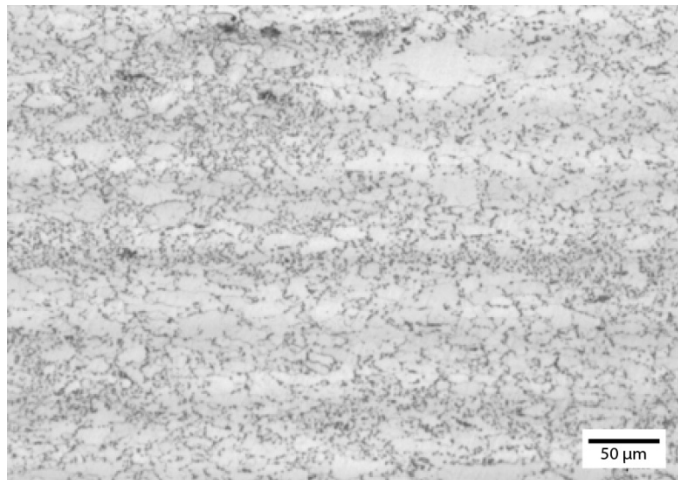
Figure 7. Micrograph of the steel after tension tested at 750°C
