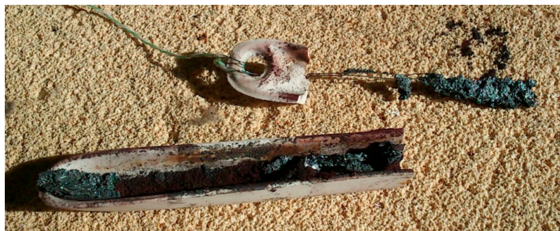
Figure 16. Sample once treated with concentrated solar energy (E20P1).
